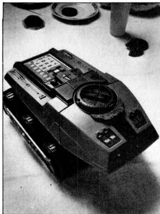
Big Trak: A tank which can be preprogrammed with details of direction, distance, pauses and the firing of 'phaser' guns.
